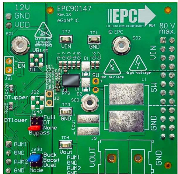
Figure 7: EPC90147 Evaluation Board (see EPC90147 Quick Start Guide for details)
